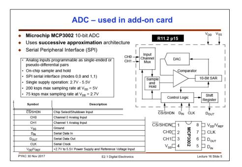
This shows the ADC block diagram. Again the digital interface obeys the SPI protocol, with Chip Select (CS), Serial Clock (CLK), Serial Data in (Din) and Serial Data Out (Dout) signals.
