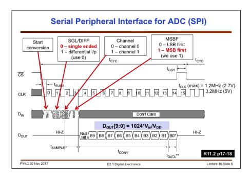
The control of the ADC is slightly more complicated than that for the DAC. Nevertheless, the idea is similar. The transfer cycle is again 16 states, going from state 0 to state 15.
